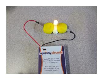
8. Now try making different shapes or adding different loads, like a buzzer motor or fan.
