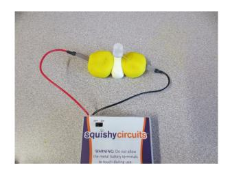
7. To complete your circuit you can now turn on the battery pack. Make sure that while your battery pack is ON, the battery leads do not touch.
