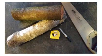
2. From the end of your material, measure and mark a line 1" from the end. – You will probably need to use a sharpie to ensure you can see the cut line.
