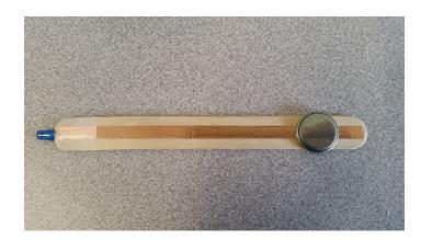
7. Secure your Battery in place using a piece of scotch tape. Be sure to only cover a portion of the battery.
