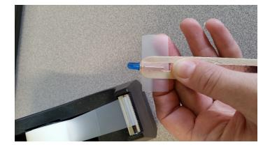
6. Collect your battery and place it on the conductive foil.
