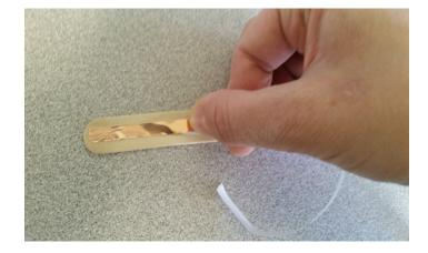
3. Smooth the conductive tape down and repeat on the back side of the stick.
